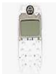
Nokia 3310 Front removed The display (with intergrated PCD8544 controller)
